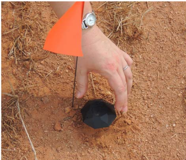
Fig. 4. Example of a soil surface being scanned using the Nix™ Pro color sensor.
