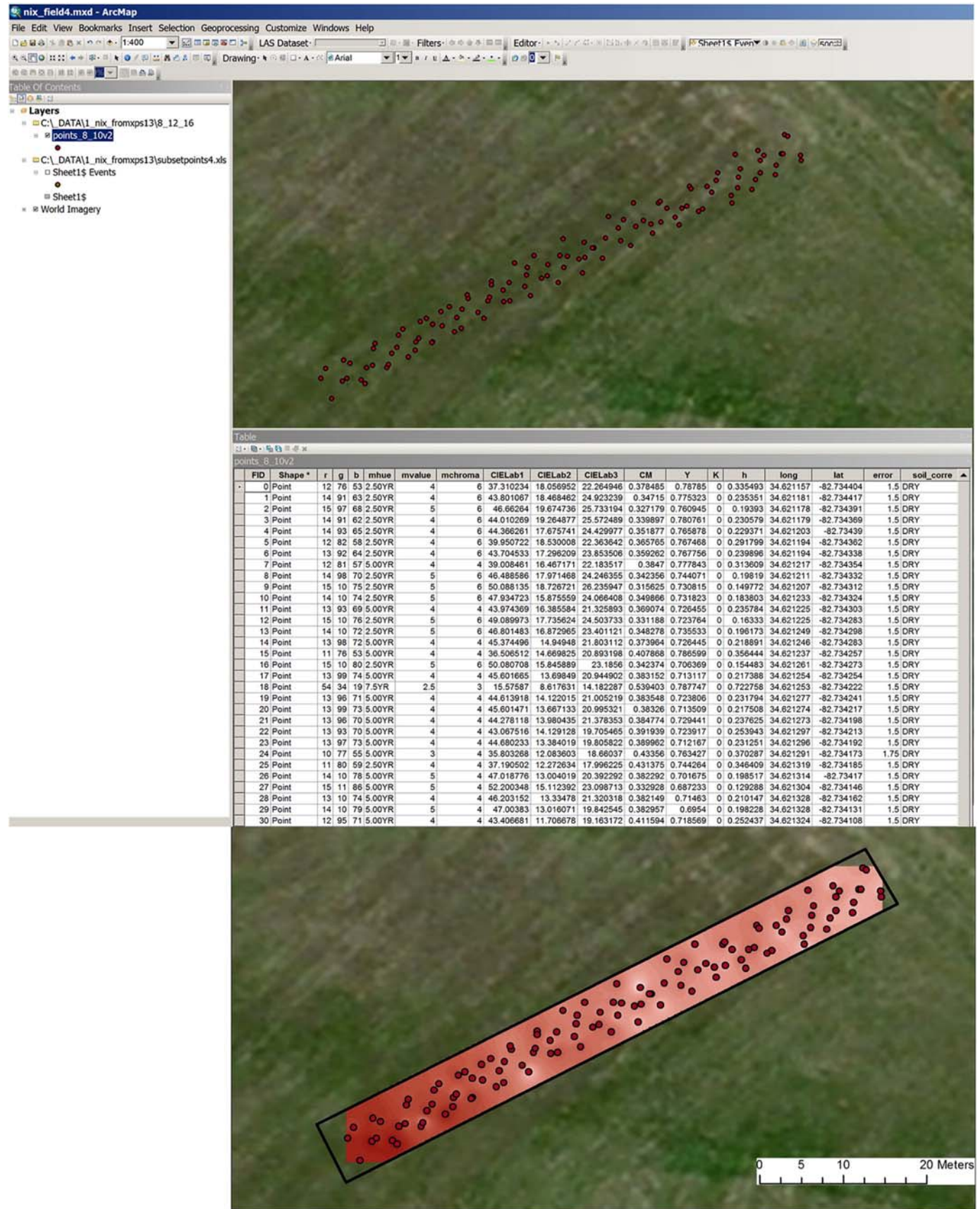
Fig. 5. GIS layouts showing: scan locations (top), soil color attributes (middle), and interpolated a* (red) color values using Inverse Distance Weighting (bottom) for the Simpson Agricultural Experiment Station.
