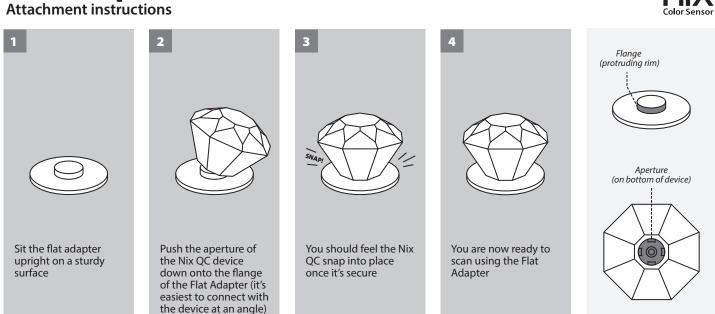
PLEASE NOTE: With the Flat Adapter attached, you may see L-values that are lower than those seen without the Flat Adapter due to light geometry. If you are using a Flat Adapter to measure your products, it is important to remember to set the master color while using a Flat Adapter as well. This way, you are comparing apples to apples. If you have any questions, please contact us at qc.support@nixsensor.com
