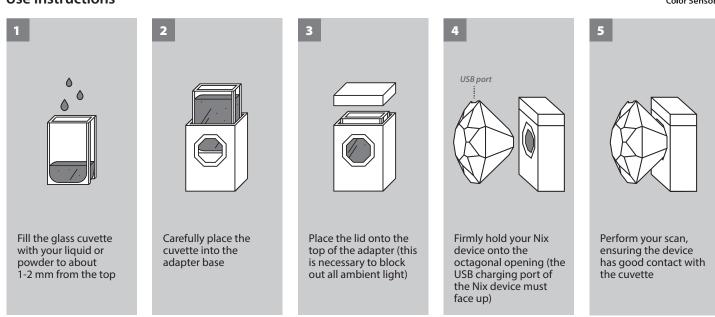
PLEASE NOTE: This adapter is measured from the **side** to elminate the formation of bubbles. Do not tip onto its back like the low-volume adapter. Keep upright at all times. If you have any questions, please contact us at qc.support@nixsensor.com
